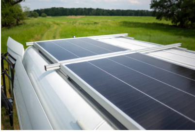
Figure 1 above depicts the basic design for our mobile charging station which we estimate to provide about 120-130 miles of total range.
